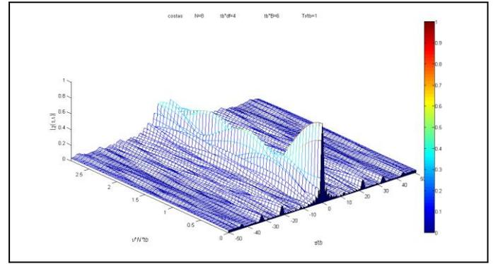
Figure 6. AF of Costas  $N=8$ ,  $t_b * \Delta f = 4$ ,  $t_b * B = 6$ ,  $T_r / t_b = 1$  at  $\tau < t_b$
