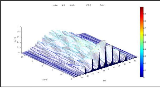
Figure 5. AF of Costas  $N=8$ ,  $t_b * \Delta f = 4$ ,  $t_b * B = 0$ ,  $T_r / t_b = 1$  at  $\tau < t_b$
